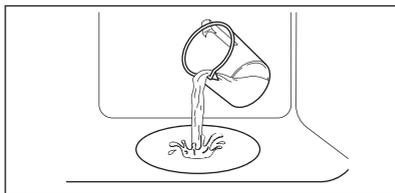
The maximum capacity of the cavity embossment is 250 ml.
