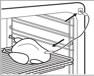
Make sure that the core temperature sensor stays in the meat and in the socket during the cooking.
