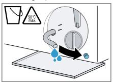
8. Firmly press on the sealing cap.
