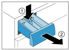
**3.** Pull out the insert upwards.
