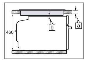
Hob type a raised in mm a flush in mm b in mm Induction hob 42 43 5 5 Full-surface induction hob 52 53 5<sup>1</sup> 43 Gas hob 32 Electric hob 32 35 2 1 Observe different national installation instructions for the hob.
