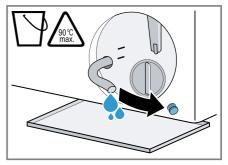
8. Firmly press on the sealing cap.
