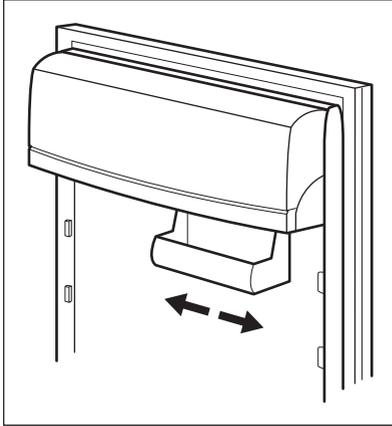
This model is equipped with a variable storage box which can be moved sideways.
