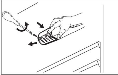
3. Replace the bulb with the one that has identical characteristics and is specifically designed for household appliances.
