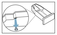
9. Turn the condensation container 180° again and insert the stopper into the recess in the top of the condensation container.
