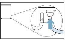
Secure the other side of the drain hose using the remaining accessories, depending on the connection situation.
