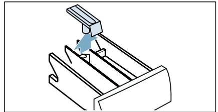
3. Clean the detergent dispenser tray and insert with water and a brush, and dry it. Clean the inside of the housing as well.
