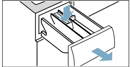
2. To remove the insert: Push the insert upwards from below with your finger.
