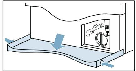
3. Take the drain hose out of the retainer.
