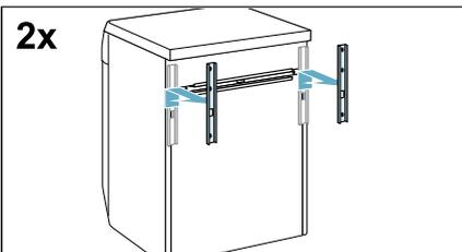
3. Undo and remove the screws on the horizontal transport strut.
