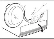
3. Turn the lever to unlock the condenser lid.
