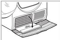
If necessary, remove the fluff from the condenser and its compartment. You can use a wet cloth and/or a vacuum cleaner with a brush attachment.
