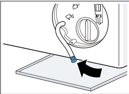
10. Insert the drain hose into the holder.
