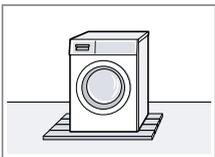
Place the appliance on a water-resistant wooden board which is screwed tightly to the floor. The wooden board should be at least 30 mm thick.
