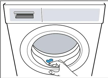
3. Leave the door and detergent drawer open so that residual water can evaporate.
