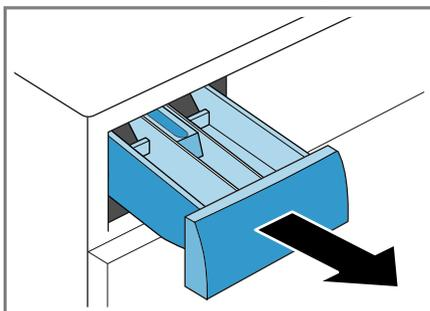
2. Press down on the insert and remove the detergent drawer.
