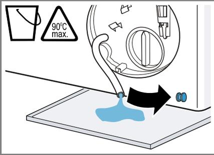
9. Firmly press on the sealing cap.
