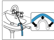
Drainage into a plastic pipe with rubber sleeve or into a gully.
