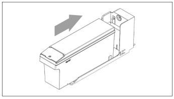
3. Refit the water storage box correctly.
