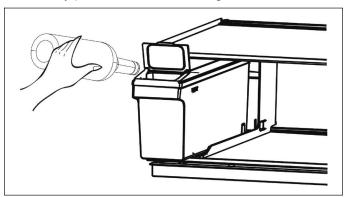
**2.** Lift the small front cover and pour in the water directly.
