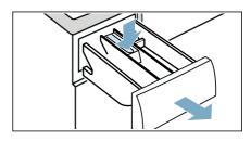
2. To remove the insert: Push the insert upwards from below with your finger.
