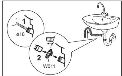
Connect the drain hose to the spigot and tighten it with a clamp. Make sure that the drain hose makes a loop to prevent particles going into the appliance from the sink.
