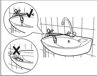
**i** Make sure that the plastic guide cannot move when the appliance drains and the drain hose end is not immersed in the water. There may be a return of dirty water into the appliance.
