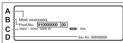
The rating plate reports the model name (A), product number (B), electrical ratings (C) and serial number (D).
