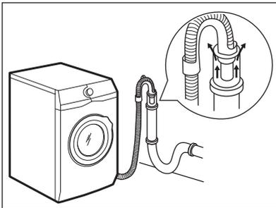
**i** The end of the drain hose must always be ventilated, i.e. the inner diameter of the drain pipe (min. 38 mm - min. 1.5") must be larger than the external diameter of the drain hose.
