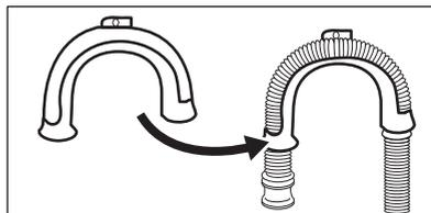
2. On the edge of a sink - Fasten the guide to the water tap or to the wall.
