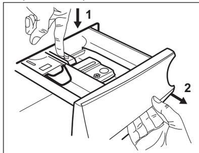
2. Remove the top part of the additive compartment to aid cleaning and flush it out under running warm water, to remove any traces of accumulated detergent. After cleaning, put the top part back into position.
