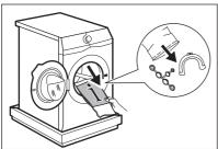
5. Remove the polystyrene protection from the bottom. Put the appliance back into an upright position.
