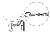
Make sure that the drain hose makes a loop to prevent particles going into the appliance from the sink.
