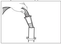
4. **To a stand pipe with vent-hole** - Insert the drain hose directly into a drain pipe. Refer to the illustration.
