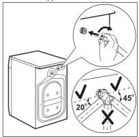
2. Position it toward left or right depending on the position of the water tap. Make sure that the inlet hose is not in vertical position.
