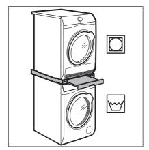
The tumble dryer can be stacked on the top of the washing machine only by using the correct stacking kit manufactured and approved by ELECTROLUX.
