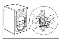
7. Remove the three transit bolts and pull out 8. Put the plastic caps, that you find in the the plastic spacers.
