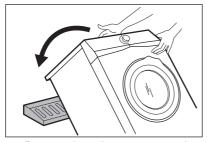
7. Remove the polystyrene protection from the bottom.
