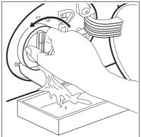
When the bowl is full of water, turn the filter back and empty the container.
