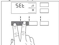
Touch related tank buttons to toggle function off and on. The display shows OFF when a tank is disabled or shows tank indicator when it is enabled.
