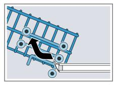
3. Re-attach the basket to the upper rollers (setting 3) or lower rollers (setting 1).
