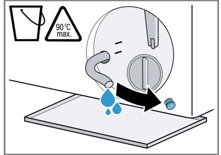
8. Firmly press on the sealing cap.
