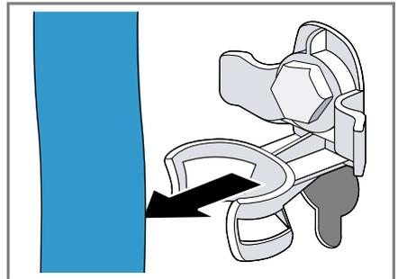
2. Unscrew ① and remove ② all screws for the 4 transit bolts with a WAF 13 wrench.
