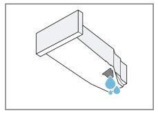
6. Insert the condensation container so that it locks into place.
