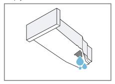
Check the condensation container filter → Page 44 regularly and clean the filter if it is dirty. Make sure that you insert the condensation container before operating the appliance.
