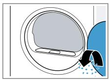
3. Remove the two-part fluff filter.
