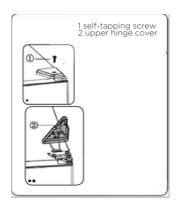
3. Remove screws 1 and hinge 2.
