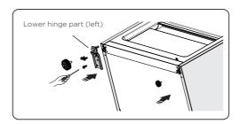
14. Slot the lower door onto the bottom hinge pin and hold in position. Turn the middle hinge by 180°, change the washer on the axis to the lower side, adjust the middle hinge to the appropriate position and then install it ensuring the lower door in secured in place.
