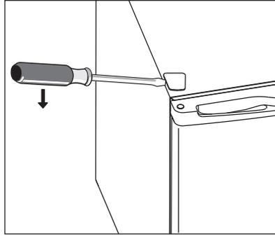
4. Move the core cover from left side to right side. And then lift the door and place it on a padded surface to prevent it from scratching.
