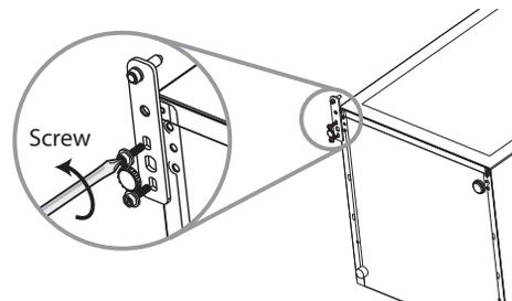
8. Place the door back on. Ensure the door is aligned horizontally and vertically so that the seals are closed on all sides before finally tightening the top hinge.
