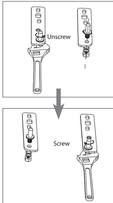
7. Refit the bracket fitting the bottom hinge pin. Replace both adjustable feet.
