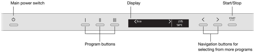
Install the dishwasher, see the chapter Installation. Following this, open the door and press the main power switch to start using the machine.
