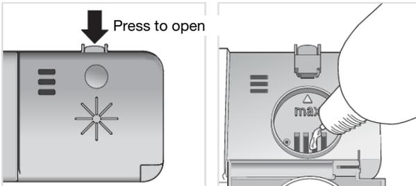
Add rinse aid to the container for rinse aid (if the dishwasher has not been connected to a system for the automated dosage of rinse aid).
