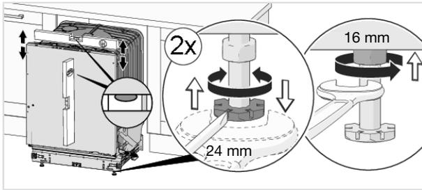
5. Check that there is an air gap of at least 3 mm between the underside of the worktop and the top edge of the dishwasher.
