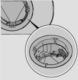
Check that the coloured stop on the right in the bottom drain is in place.
