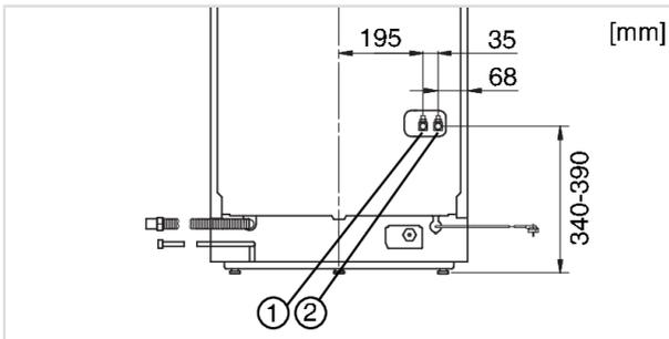
1. *Connection for detergent (hose diameter 6 mm). Remove the plug and connect the hose.*
