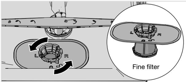
1. Turn the locking ring anticlockwise and lift the fine filter straight up.
