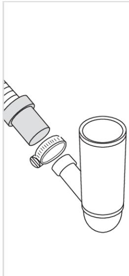
The drainage hose can also be connected to a connection nipple on the sink unit's water trap. The connection nipple must have an internal diameter of at least 14 mm.
