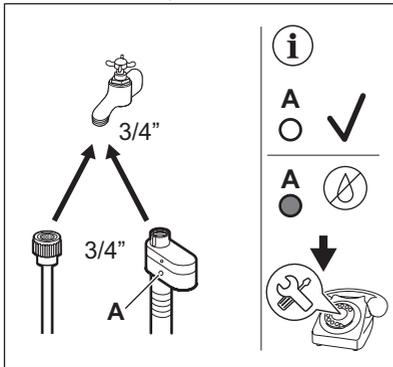
5. Connect the other end of the COLD water inlet hose to the cold water tap with 3/4" thread.
