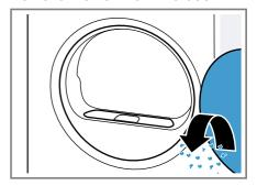
3. Remove the two-part fluff filter.
