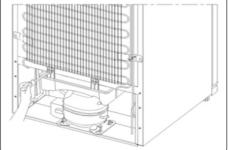
Remove the vaporisation container from its position by removing the screws as indicated. Clean it with soapy water at specific time intervals. This will prevent odours from forming.
