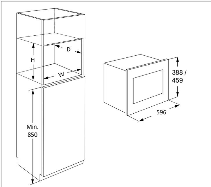
The microwave can be fitted in position A or B:
