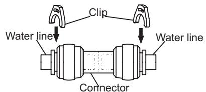
Open the water valve to flush the lines, and check leakage in the water connectors. If any leak, please check that if the lines are fully inserted where the connector leaked. If not, please install them again, and make sure that the lines are fully inserted.
