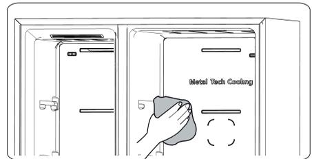
Although this appliance automatically defrosts, a layer of frost may occur on the freezer compartment's interior walls if the freezer door is opened frequently or kept open too long. If the frost is too thick, choose a time when the freezer is nearly empty and proceed as follow:
