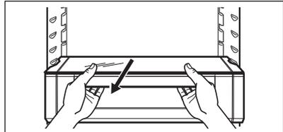
2. Tilt the module downwards to remove it from the refrigerator.
