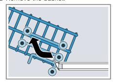
Re-attach the basket to the upper rollers (setting 3) or lower rollers (setting 1).
