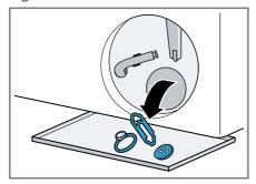
**3.** Ensure that both impellers can turn.
