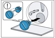
The pump cap is comprised of two parts which can be taken apart for cleaning.
