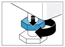
To align the appliance, turn the appliance feet. Check that the appliance is level using a spirit level.
