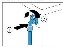
3. Connect the water inlet hose to a tap (26.4 mm = 3/4").
