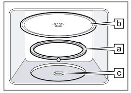
**3.** Check whether the turntable is correctly engaged. Note: The turntable can turn anti-clockwise or clockwise.
