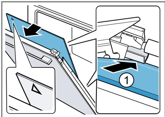
✓ The intermediate pane is automatically positioned by the rotational movement of the spacer.
