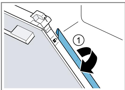
8. Pull the first and second intermediate panels upwards and out at an angle, and set them down carefully on a flat surface.
