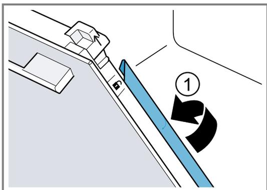
4. Slide the inner panel into the retainer at the bottom ① and fit it at the top.
