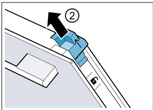
6. Remove the inner panel upwards at an angle and set it down carefully on a flat surface.
